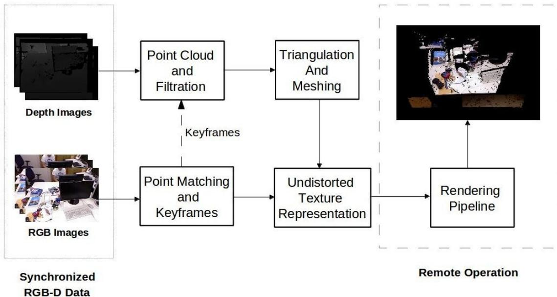
Figure 1: Overview of our approach. The input to the system is depth image sequence (or point clouds) and synchronized RGB images. The output is 3D reconstruction of the environment which is efficient in computing, storage and capable to apply in real time
