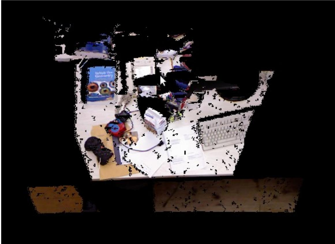
*Figure 2: Result of 3D scene reconstruction from a single view by using downsampled data from RGBD sensor.*
